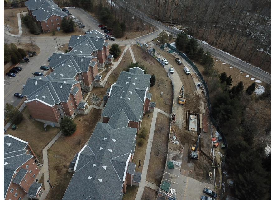
Aerial view of Equalization Tank Installation on Husky Circle
