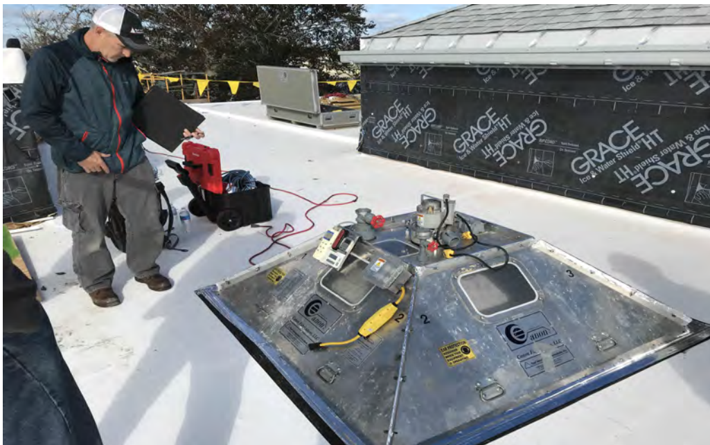
Uplift testing at new PVC roof
