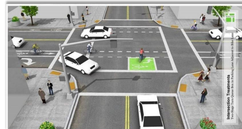
At a signalized intersection with two-stage turn queue boxes, PTV riders need to receive two separate green signal indications to turn, and at unsignalized intersections, PTV riders need to wait for appropriate gaps in crossing vehicular traffic. Green pavement and bike symbols are used to designate the queue boxes. It is important to note that the FHWA issued an Interim Approval in 2017 for the use of two-stage bicycle turn boxes
