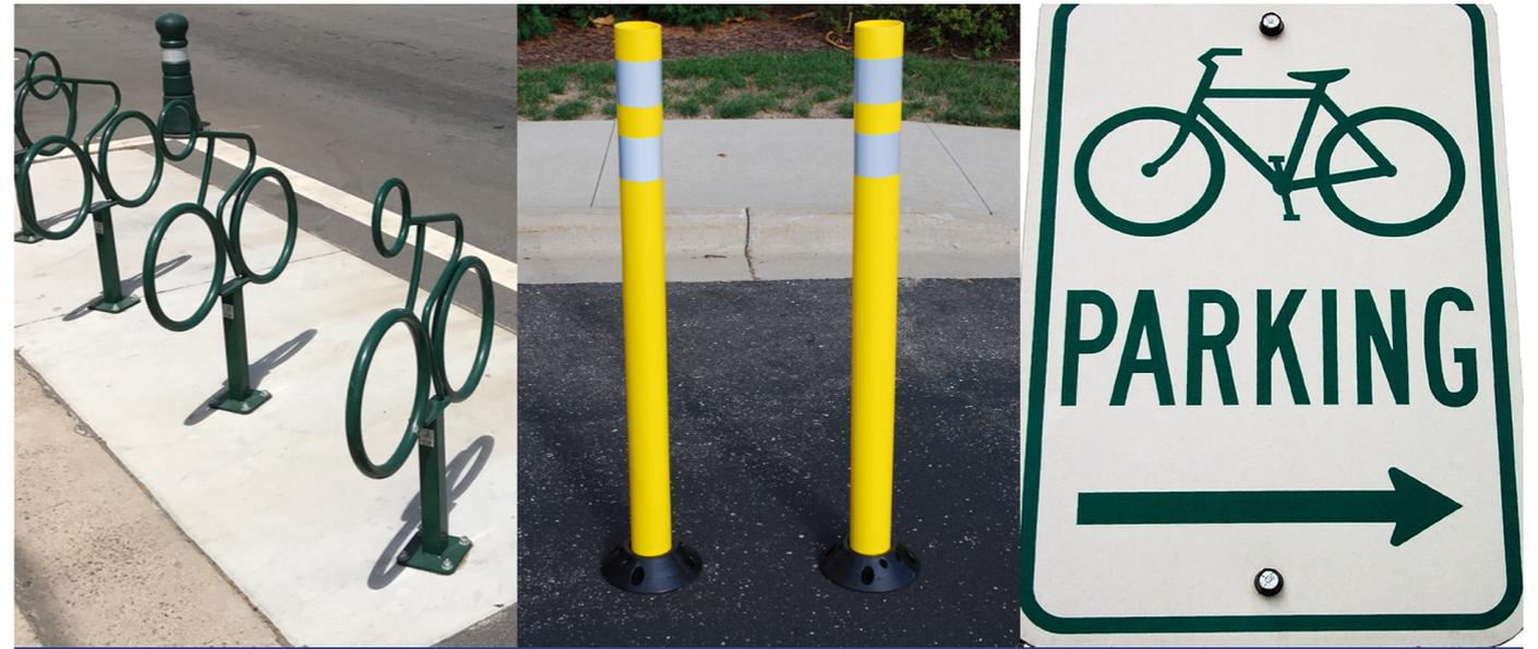
Signs, delineators and markings on the ground are ways to help cyclists easily locate and access bike parking areas.
